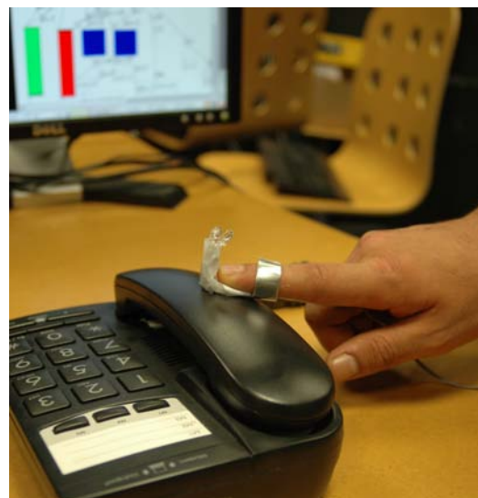
Figure 1: A phone used as an opportunistic fader to control a sound parameter.
